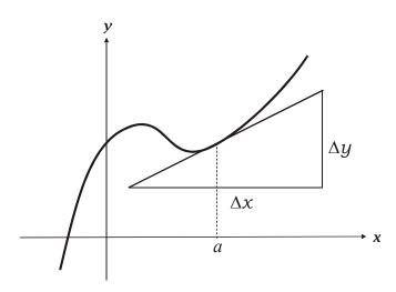
As the diagram indicates, the gradient can be found by graphical means.
