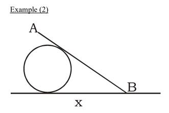
A uniform rod AB, of length 18a and mass 2m leans against a cylinder. Its base B is hinged to a rough floor. The whole system is in static equilibrium. there is no friction between the rod and the cylinder, but the contact between the cylinder and the floor is rough. The angle made by the rod with the floor is  $2\theta$  where
