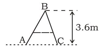
A step-ladder is made of two metal pieces, AB and BC. The length of AB is 3.9m and that of BC is 3.75m, when open the height of the ladder is 3.6m above the ground. The metal pieces are modelled as uniform rods and they are smoothly hinged at B. The floor is smooth and the distance AC = 2.55m. The two metal parts are joined by a light horizontal rope of length 1.7m. The weight of AB is twice that BC. If the tension in the rope is 12.25N find W.
