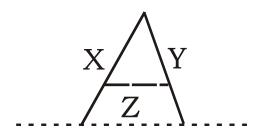
The ladder comprises two metal pieces X and Y, hinged together and standing on a smooth floor, held together by a rope, Z. Y is shorter than X. Since the floor is smooth there are no frictional forces at the floor, consequently there are only the normal reactions to consider at the floor. In this illustration we shall also suppose that both vertical pieces, X and Y, have the same weight W.
