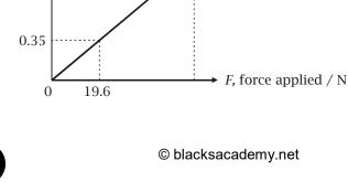
We cannot carry on this graph beyond an extension of 1.50 m because after that point the spring is deformed.
