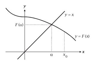
The diagram shows the graph of y = F(x) and y = x and the initial approximation,  $x_0$ . At the point of intersection, where  $x = \alpha$ , we have  $F(\alpha) = \alpha$ , hence  $g(\alpha) = F(\alpha) - \alpha = 0$ . So this is a solution of g(x) = 0. The value of the first approximation is shown in the following diagram.
