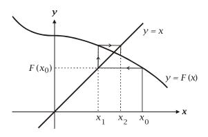
However, when the gradient of y = F(x) is greater than 1 around the root  $\alpha$ , then the series of successive terms generated by the method diverges away from  $\alpha$ , as the following diagram illustrates
