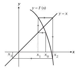
So for the method to work we must have |F'(x)| < 1. Furthermore, the rate of convergence is faster, the smaller |F'(x)| is.
