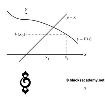
At the point of intersection  $y = F(x_0)$  with y = x we have the value of the second approximation,  $x_1$ . The following diagram shows how repetition of this process causes successive approximations to converge on the root  $\alpha$ .
