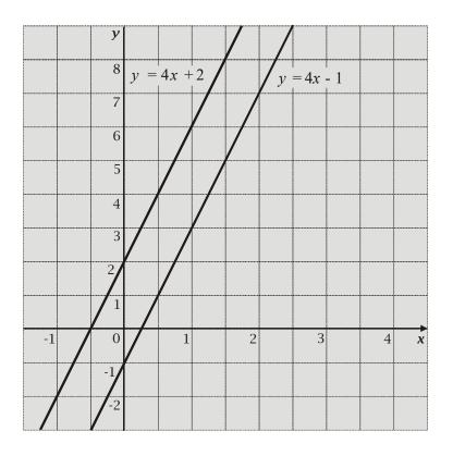
These two lines are parallel. They have no simultaneous solution.
