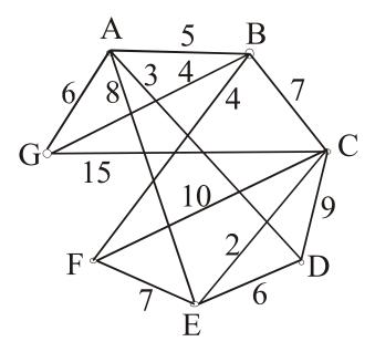
(a) We shall find a minimum connector of the graph shown above using Prim's algorithm.
